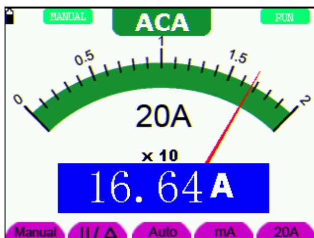
figure 30: AC Current Measurement for 20A
