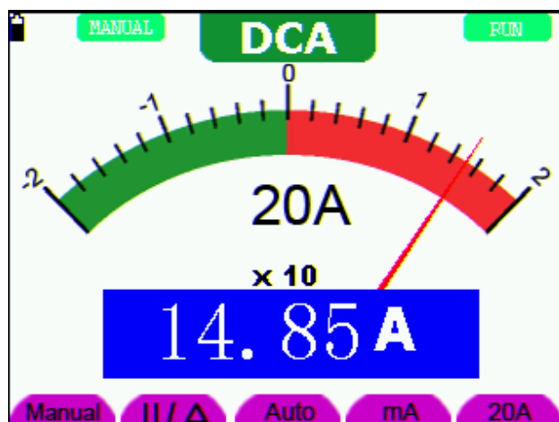
figure 28: DC Current Measurement for 20A
