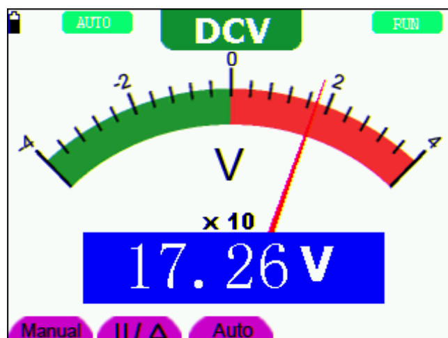
figure 25: DC Voltage Measurement
