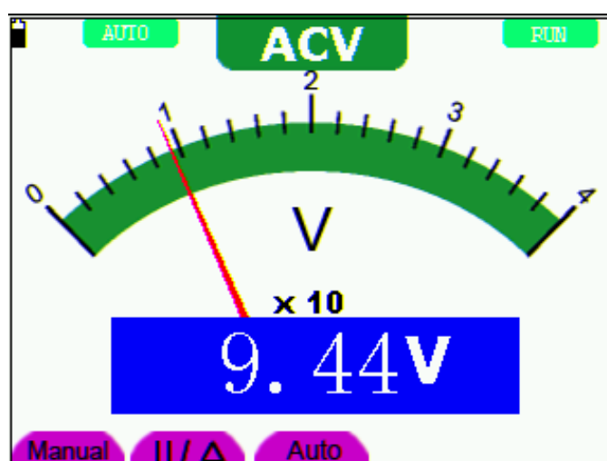
figure 26: AC Voltage Measurement
